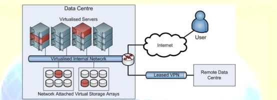
Connectivity between data centres owned by a single provider is implemented by leased virtual networks providing guarantee, but static quality of service for the IaaS owner.
